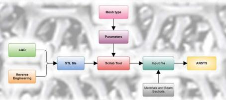
The tool implemented in Scilab allows to read the STL file and, choosing the parameters for the definition of the elementary cell, generates the array of the structure. Then the intersections between a surface and the array are calculated by the ray tracing technique and is written an input file for Ansys with the information to be used in FEM analyses.
